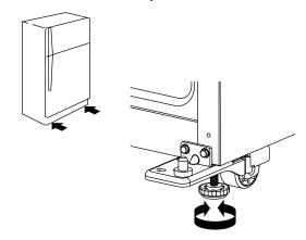
Open both doors again to make sure they close as easily as you like. If not, tilt the refrigerator slightly more to the rear by turning both leveling legs to the left; it may take several more turns.
