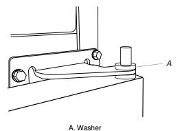
Using a hex-head socket wrench and an open-end wrench, remove the three screws from the center hinge and remove the hinge. Set aside.
