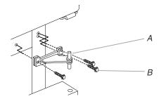
A. Center hinge B. <sup>5</sup>/<sub>16</sub>" Hex-head hinge screws
